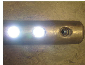
Two powerful LED lights seen in the water cooled camera. Only a 50mm large opening is needed for access.
